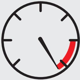
KELLER pressure sensors, transducers and transmitters are designed to withstand a certain amount of overpressure without damage or calibration shift. It can range from 15X for the lower pressure ranges to 1.1X for the highest ranges. This value is different for each product and is referred to in the literature as “Overpressure.” Also found in the literature is usually a value for “Burst Pressure,” which is the pressure at or above which there may be catastrophic failure of the product.
