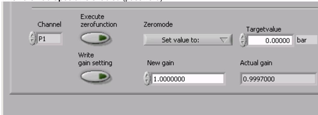
Channels CH0, P1 and P2 of the digital-transmitter have a linear gain and an offset:
