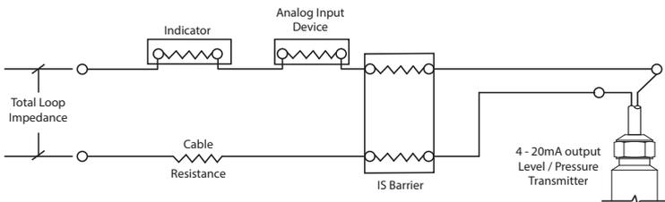
The calculations below are useful in identifying the minimum supply voltage needed for a current loop with additional line impedances or conversely, the maximum current loop impedance allowed for a given supply voltage.
